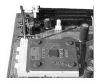
Step 3 Close the socket by closing the tuation lever.
